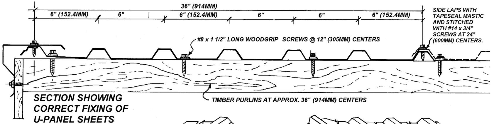
NOTE: AT ALL EDGES OF ROOF FASTEN SHEETS TO PURLIN AT 6" (152MM) CENTERS.
